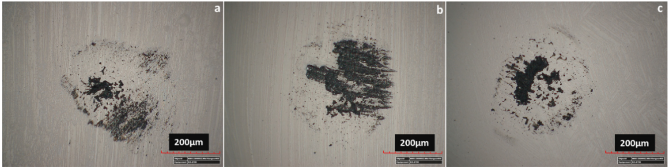
Fig. 5. Optical microscope surface of testing alumina balls after the dry sliding friction test. (a) Electroless NiB without ultrasound, (b) electroless NiB with 20 kHz frequency and 0.058 W/cm 3 energy density ultrasound, (c) electroless NiB with 35 kHz frequency and 0.065 W/cm 3 energy density ultrasound.
